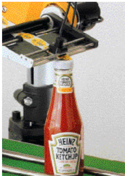
High-precision labeling accuracy: Collamat® 3600 offers a labeling accuracy of \pm 1 mm. ( \pm 1/25 in)
